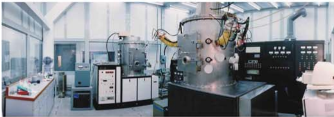
Fig. 1. Class-1000 cleanroom housing the multi-purpose plasma immersion ion implanter in the foreground and semiconductor PIII machine in the background.
