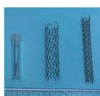
Fig. 4. PIII Treatment of blood vessel stents to improve x-ray
