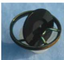
Fig. 2. Artificial heart valve treated by PIII in the Plasma Laboratory.
