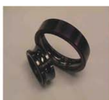
Fig. 3. PIII treatment of the races of the inner and outer rings of a satellite ball bearing.
